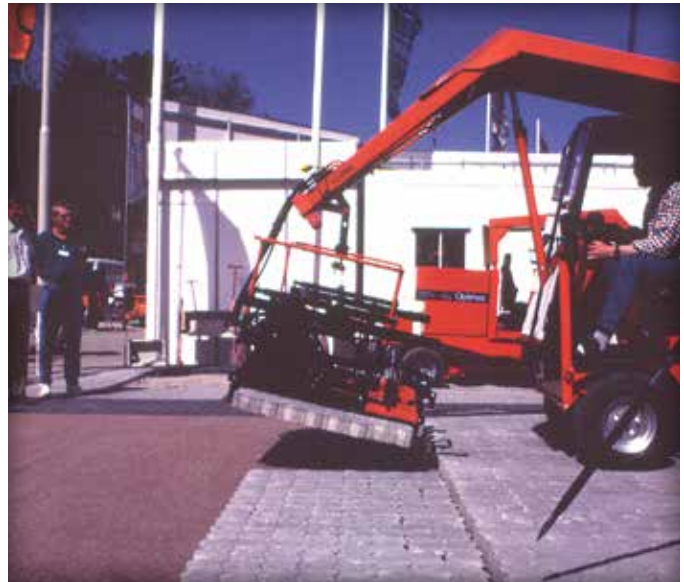
Figure 21. After the layers are separated they can be grabbed by the machine clamp.
